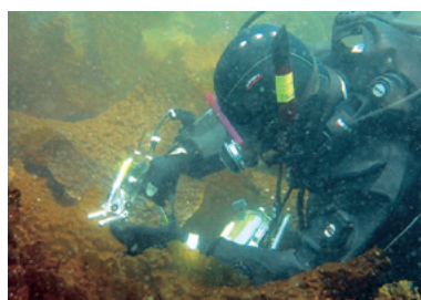
Diving-PAMを用いた海藻の光合成の水中測定 Underwater Measurement of Some Algae by Using Diving-PAM
